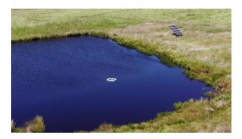
Figure 3: Solar powered submersible pump. Photo: South East Local Land Services
